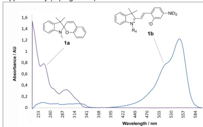
**Figure 2.** Representative absorption spectra of **1a** and **1b** recorded at a concentration of 10  $\mu\text{M}$  in methanol in a 10 mm light path cuvette at ambient temperature after 30 min of dark adaptation.
