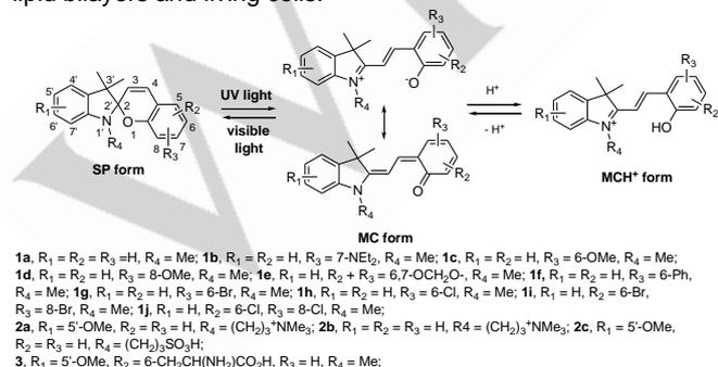
**Figure 1.** Overview of the photoisomerization and acidochromism of spiropyrans, the model spiropyran-derived compounds studied in this work.
